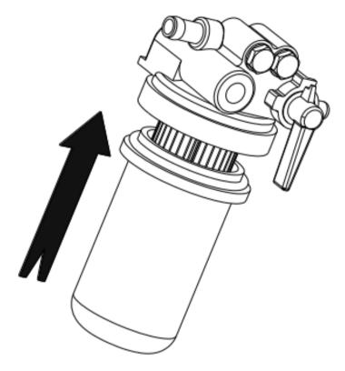
Install the casing bowl (1) fitted with an Oring seal (5) over the filter. Seal should be seated against the base (1).
