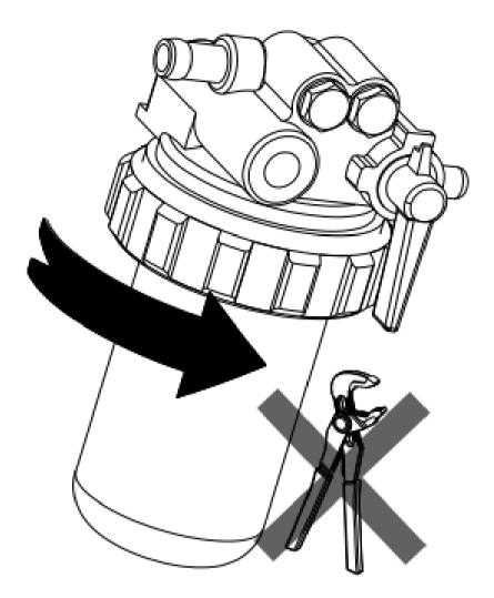
Position the locking ring (3) over casing bowl (4). Take special care in aligning threads and screw on the locking ring finger tight. Ring should turn freely when threads are properly engaged. Tighten the locking ring (4) hand tight. DO NOT USE PLIERS OR ANY OTHER TOOL TO TIGHTEN THE RING. OVERTIGHTENING THE LOCK RING CAN DAMAGE THE FUEL FILTER ASSEMBLY AND CAUSE FUEL LEAKAGE.
