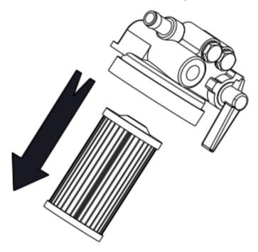
Remove the filter element (2) from the assembly by pulling it downwards. In the event that metal flanges separate from the filter element, ensure they are removed as well.
