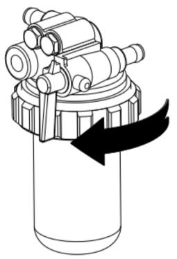
Loosen the locking ring (2) by twisting it in the indicated direction. If the ring is seized use pliers to remove it. Do not use excessive force to remove the lock ring to prevent damage. While supporting the casing bowl (4) against the base (1) to prevent fluid leakage, slip off the locking ring to remove it from the assembly.
