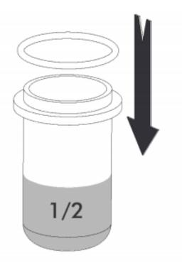
Install the O-ring seal (5) over the casing bowl (4). Seal should have a tight fit, if loose replace the O-ring seal. Fill the casing bowl (4) with clean diesel fuel no more than half way. Insert a new filter element (2) up into the base (1). Ensure the central opening of the filter is firmly pressed against the base. When installed correctly filter should hang from the base on its own.
